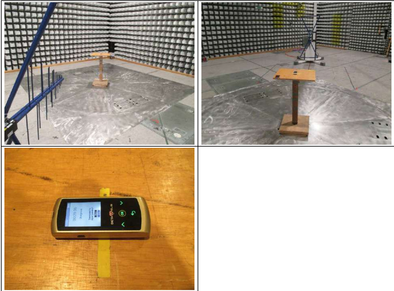
Figure 6-5: test setup for Radiated disturbances 30 MHz to 1000 MHz
